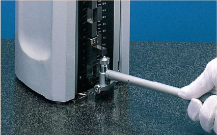
Bore gage zero-setting
